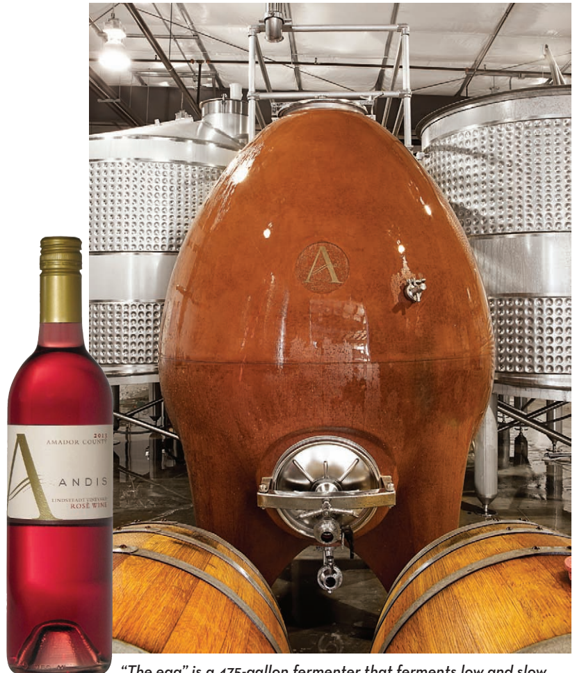
“The egg” is a 475-gallon fermenter that ferments low and slow.
